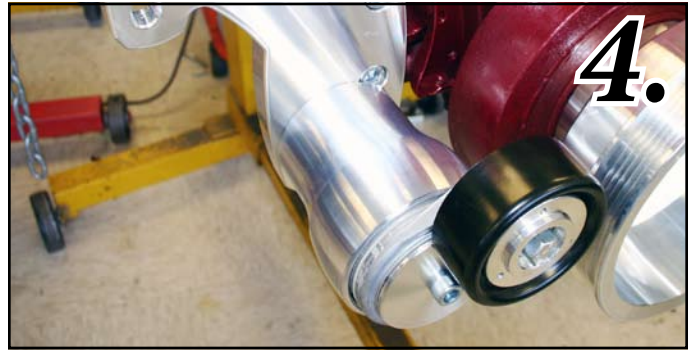
Photo-5 Mount the power steering Spacer Bracket (20357-B) & Power Steering Housing Cover (20357-C) and the power Steering pump together using (2) M8 x 1.25 x \frac{3}{4} " SHCS.
